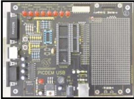
**Photo 7**—If you prefer an assembled alternative to the PICProto USB, the Microchip PICDEM USB provides the basic functionality of the PICProto USB in addition to the ability to experiment with using USB to control an LCD and game pad. The PICDEM USB LEDs, which can be switched out with a jumper or at the firmware level, illuminate to signal each state of enumeration.
