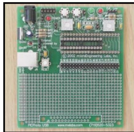
**Photo 3**—All of the goodies that complement the everyday PIC are included with this board. There are a couple of potentiometers, a pair of LEDs, and two push-button switches. The 25-pin connector pad layout suggests that a serial-to-USB thing could happen in the prototype area.
