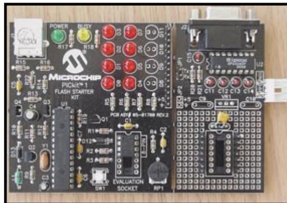
**Photo 1**—The PICkit 1 Flash starter kit is designed to program and read the new 14-pin flash memory PICs and the legacy 8-pin flash memory parts. The PICkit 1 comes with an extensive software and firmware library that includes source code for the host and PIC USB interface. I populated the snap-off part of my PICkit 1 with a Sipex SP232ACP and supporting components.
