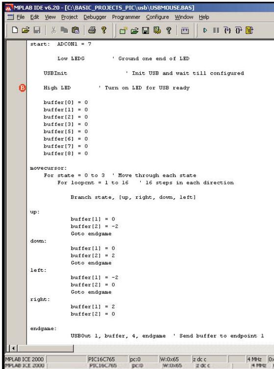
**Photo 4**—I wanted to show you the `USBInit` instruction and the MPLAB ICE 2000 breakpoint. Now you should have an idea of how PicBasic Pro fits inside an MPLAB IDE session. Note that only two PicBasic Pro USB commands are used, `USBInit` and `USBOut`.
