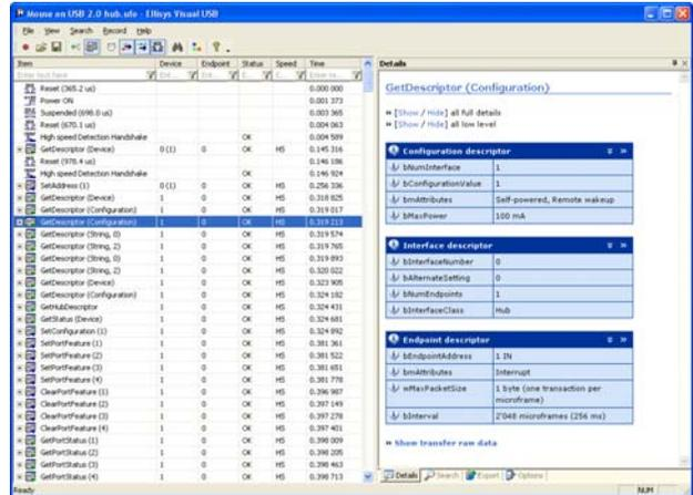
A second window gives more details. To make it easier to identify packets, the system's software includes filtering and packet-coloring functions. It also lets you select levels of detail. Also, the information derived from bus traffic is equated with references to the USB standard.
