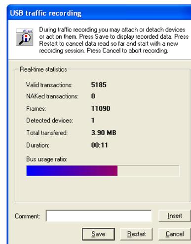
Note that the USB Tracker's real-time recording and analysis capability relies on a USB 2.0 connection. As such, the vendor notes that two host controllers comprise an optimum set-up. The first controller is used to connect the peripheral to be tested, and the other controller is used to record your data.
