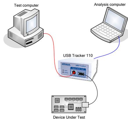
In any case, the USB Tracker's PC executables run under either Windows 98, Windows SE, Windows Me, Windows 2000, or Windows XP on PCs running Pentium IIIs clocking at least 600 MHz, with at least 128 Mbytes of DRAM. You should also equip your PC with a USB 2.0 host controller (for 480 Mbits/s operation).
