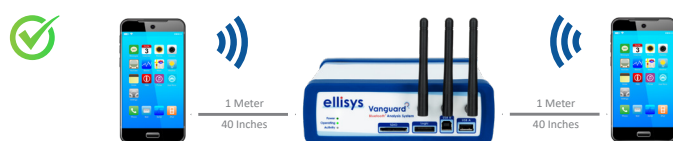
Figure 1 Analyzer Positioning Set-up
