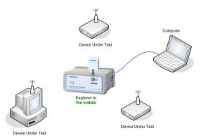
If the WiMedia Explorer 300 is not placed at an equal distance from the transmitting units, this may result in causing transmission issues that are not related to the Devices Under Test:
